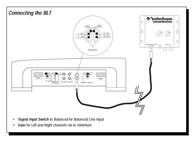
CAUTION!! You must turn the gain controls to minimum when using the Balanced Line Transmitter. If the input gains need to be adjusted, this can now be done in the Balanced Line Transmitter.
